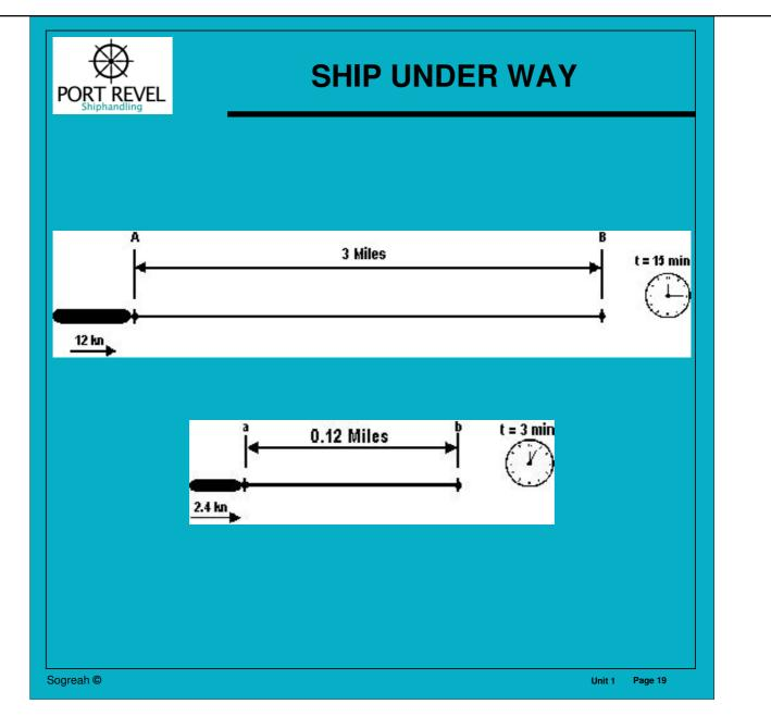
To illustrate the application of these various scales, we shall consider a 190,000 DWT **ship under way** maintaining a constant full speed of 12 knots at 65 r.p.m. (Fig. 2). It will thus cover 3 miles (about 18 ship's lengths) in 15 minutes.
