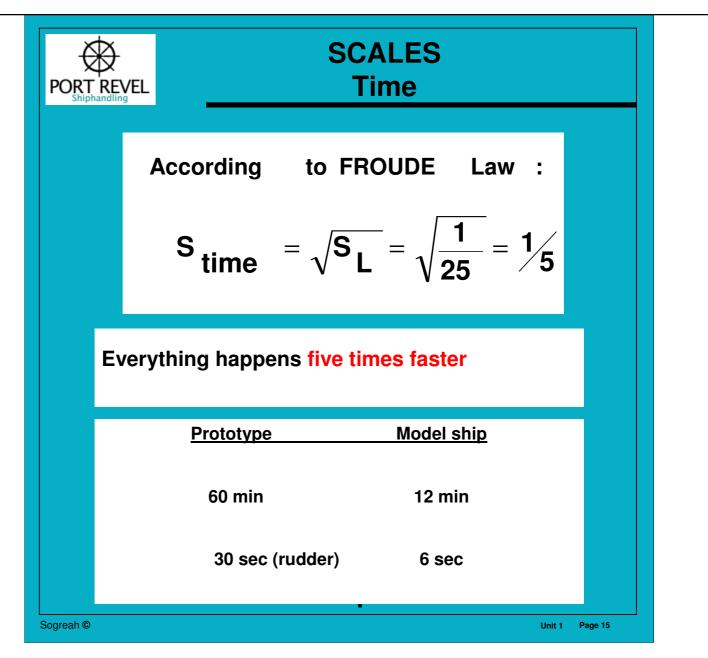
As the velocity scale is the square root of the length scale (according to Froude's law) the **model motions are five times slower** than the real thing, and, consequently, time is five times shorter than in nature.
