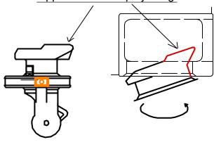
Insert upper fixed cone projecting into corner fitting and turn to counterclockwise. And then twist lock is automatically locked by locking mechanism.
