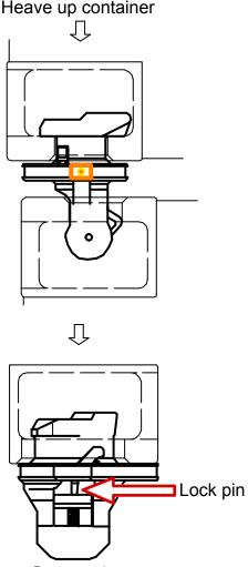
Pushing lock pin to left, turn twist lock clockwise.
