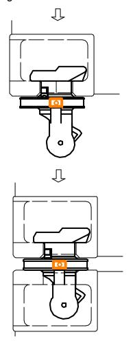
After stack container twist lock is locked automatically.
