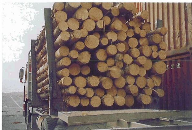
Figure 1 The JAS volume of this load of logs is about 30% less than true cubic.
